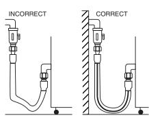
connections must avoid sharp bends that may restrict the flow of gas to the appliance. If the connected pressure exceeds 14.0" W.C. (3.5 kPa), a step-down regulator is required to be supplied by the owner/operator.
